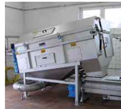
Reliable faecal sludge acceptance system – the HUBER Sludge Acceptance Plant RoFAS.
