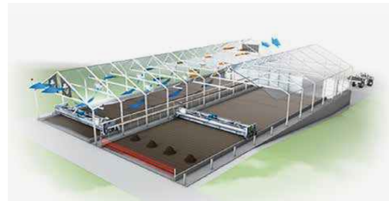
Dewatered sewage sludge becomes dry, stable sludge granulate.
