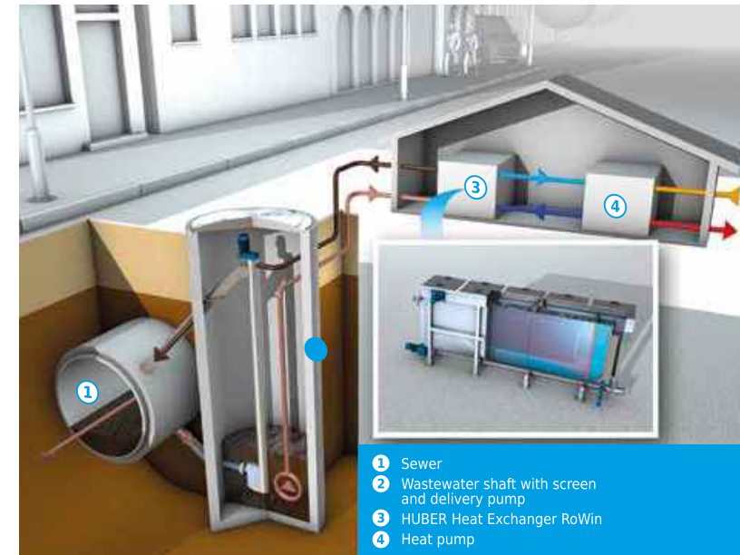
Schematic diagram of heat recovery from raw sewage by means of an above ground installed HUBER ThermWin system.
