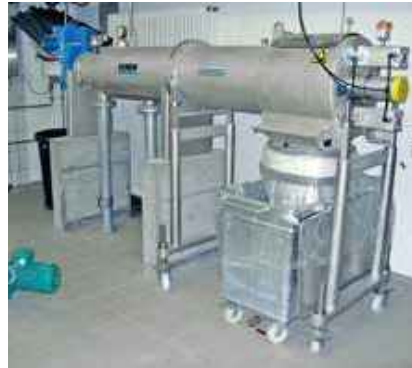
HUBER Sludg cleaner STRAINPRESS® – continuous pressurised coarse material separation.
