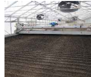
Dewatered sewage sludge becomes dry, stable sludge granulate.
