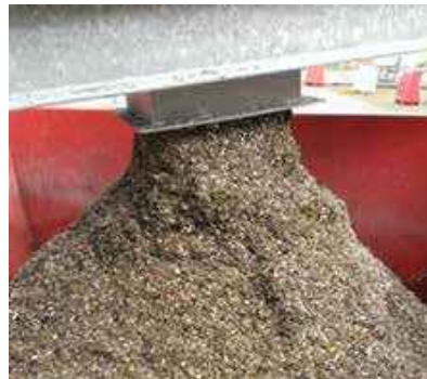
Plastics separated by fermentation residue screening.
