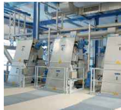
HUBER Multi-Rake Bar Screen RakeMax® – robust design for reliable operation.
