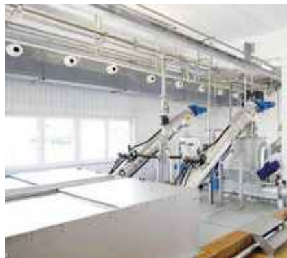
HUBER Rotary Drum Fine Screen ROTAMAT® Ro2 with up to 3 m screen basket diameter.
