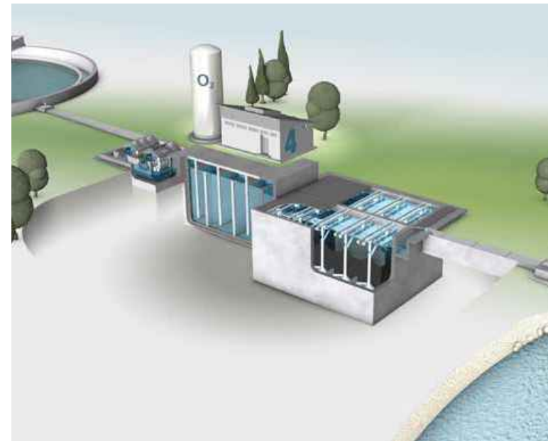
Advanced wastewater treatment for removal of trace substances with the combined process of ozonation and downstream HUBER Activated Carbon Filter CONTIFLOW® GAK.
